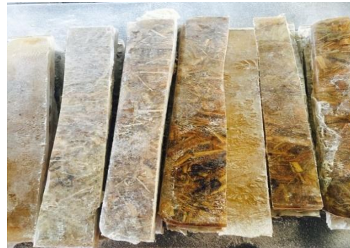
Fig.2 specimen for impact test
