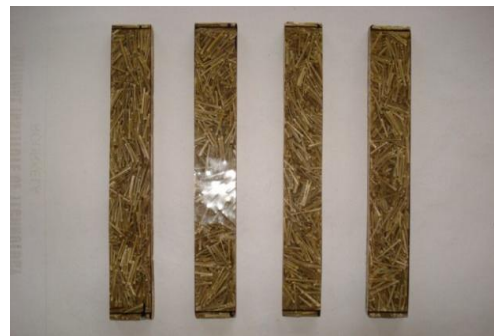
Fig.4 Specimen for Flexural test
