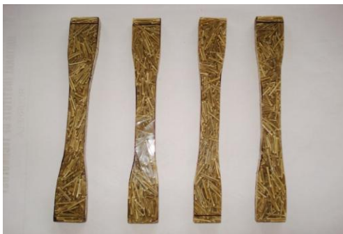
Fig.3 Specimen for Tensile test
