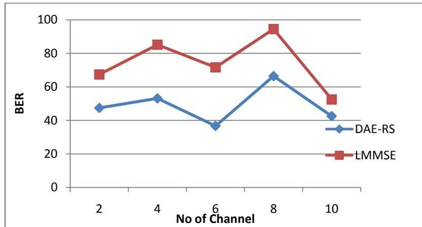
Figure. 3 BER Vs channel
