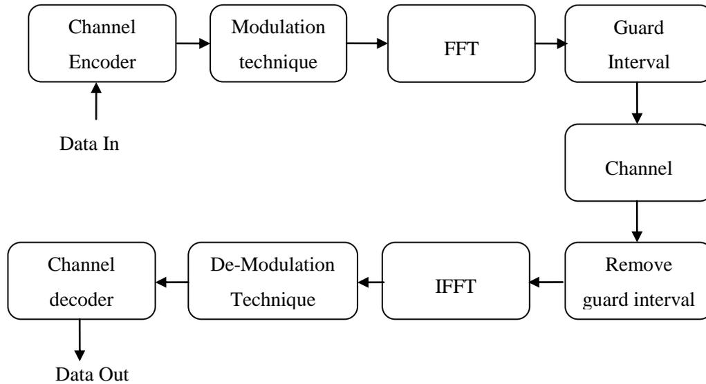
**Figure. 1. OFDM Architecture**
