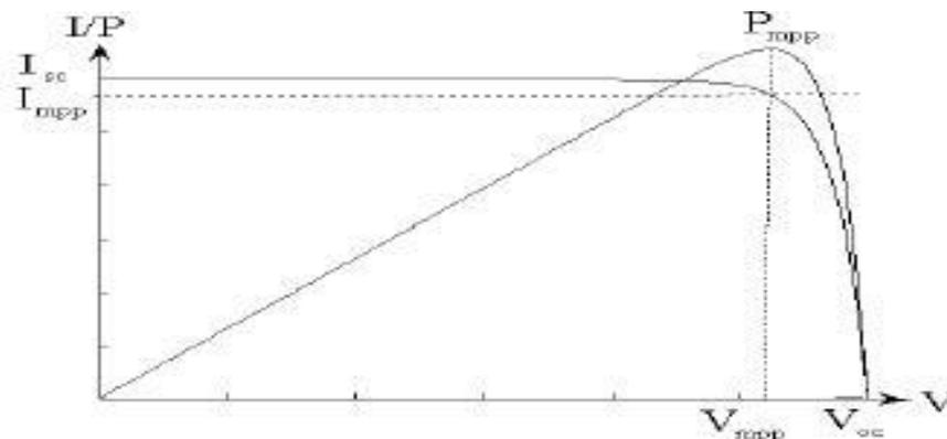
Fig 1. *I-V* and *P-V* characteristics of photovoltaic cell
