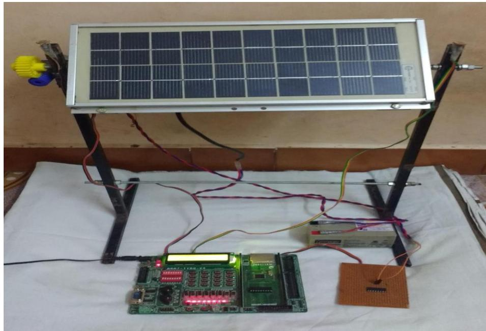
**Fig 3. Real View of Solar Tracking System**
