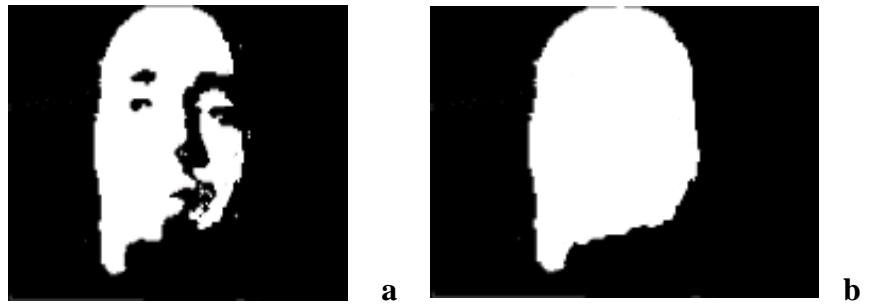
Fig 5 a. Result of thresholding and majority filter b. Morphological processing output
