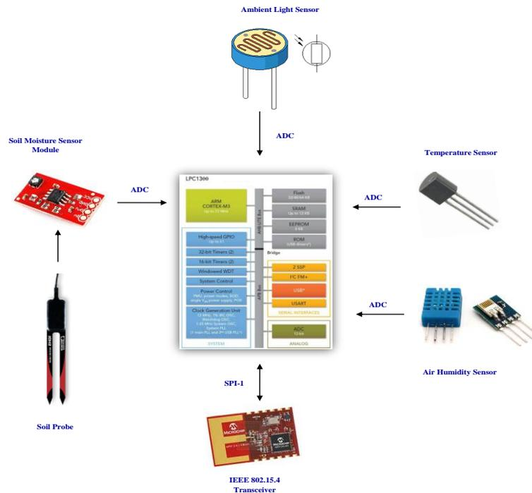
Figure 1: Wireless Sensor Node
