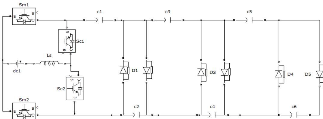
**Figure 2:** Proposed DC-DC converter
