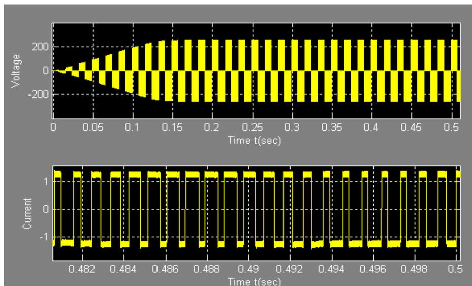
**Figure 5:** Output Voltage and Current Waveform for R Load Condition
