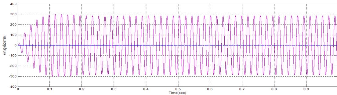
**Figure 6:** PFC output shows voltage and current in phase
