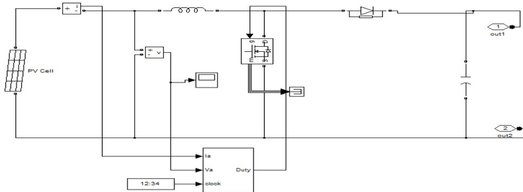
**Figure 4:** PV DC-DC boost converter
