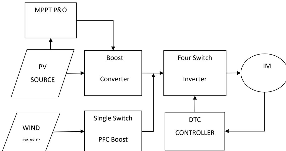
**Figure 1:** Block Diagram of Proposed multi-port converter fed Induction motor drive
