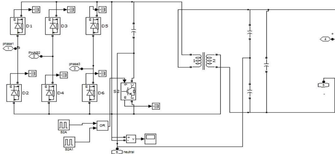
**Figure 3:** Circuit Diagram of PFC single switch-based boost rectifier
