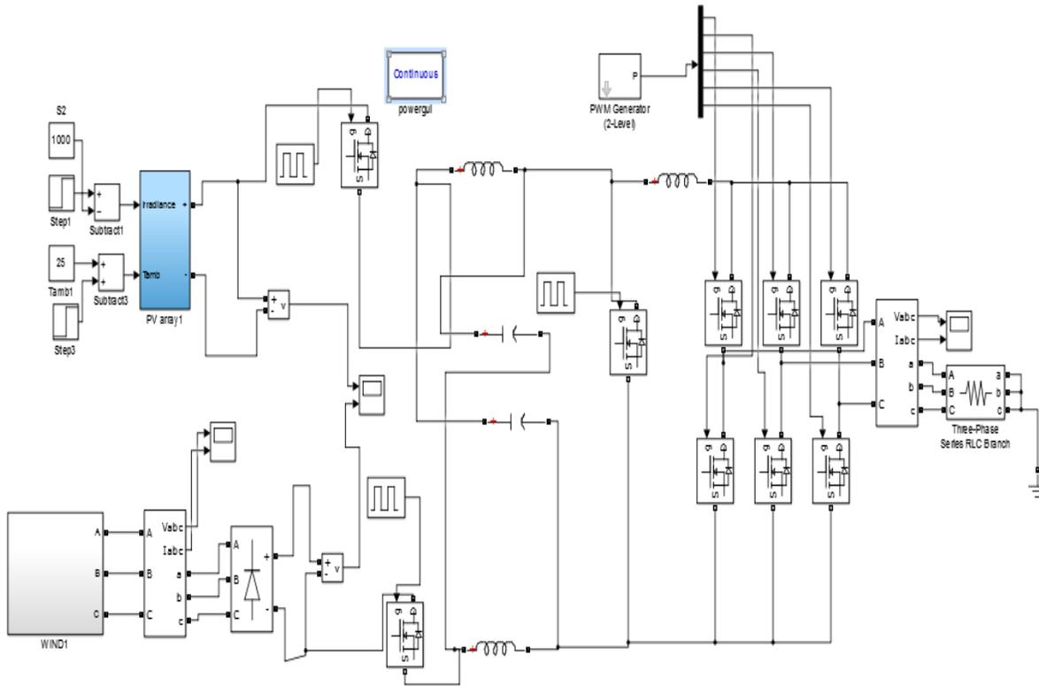
**Figure 4:** Proposed solar and wind-based Z source inverter
