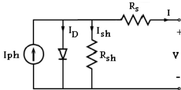
Figure 1: Single diode PV model
