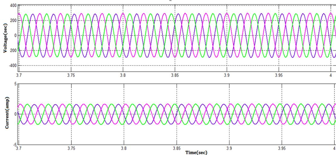
**Figure 7:** Voltage and current waveform of Z source inverter
