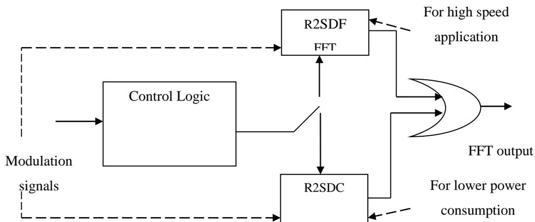
**Figure 1. Adaptive FFT Process**
