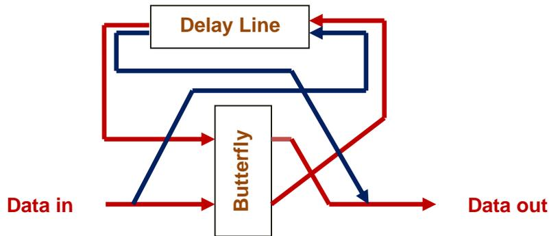
**Figure 2:** Butterfly structure for R2SDF FFT
