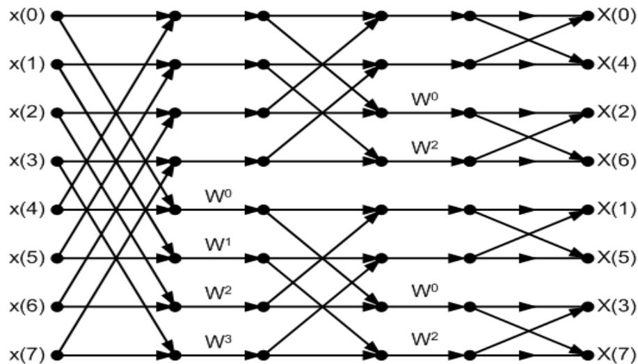
Figure 1: Radix-2 DIF-FFT structure for 8-point
