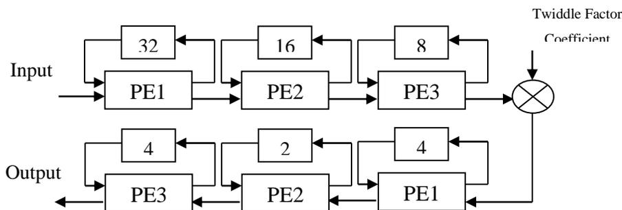
**Figure3.** Radix-2 Single-path Delay Feedback FFT with Modified BPM
