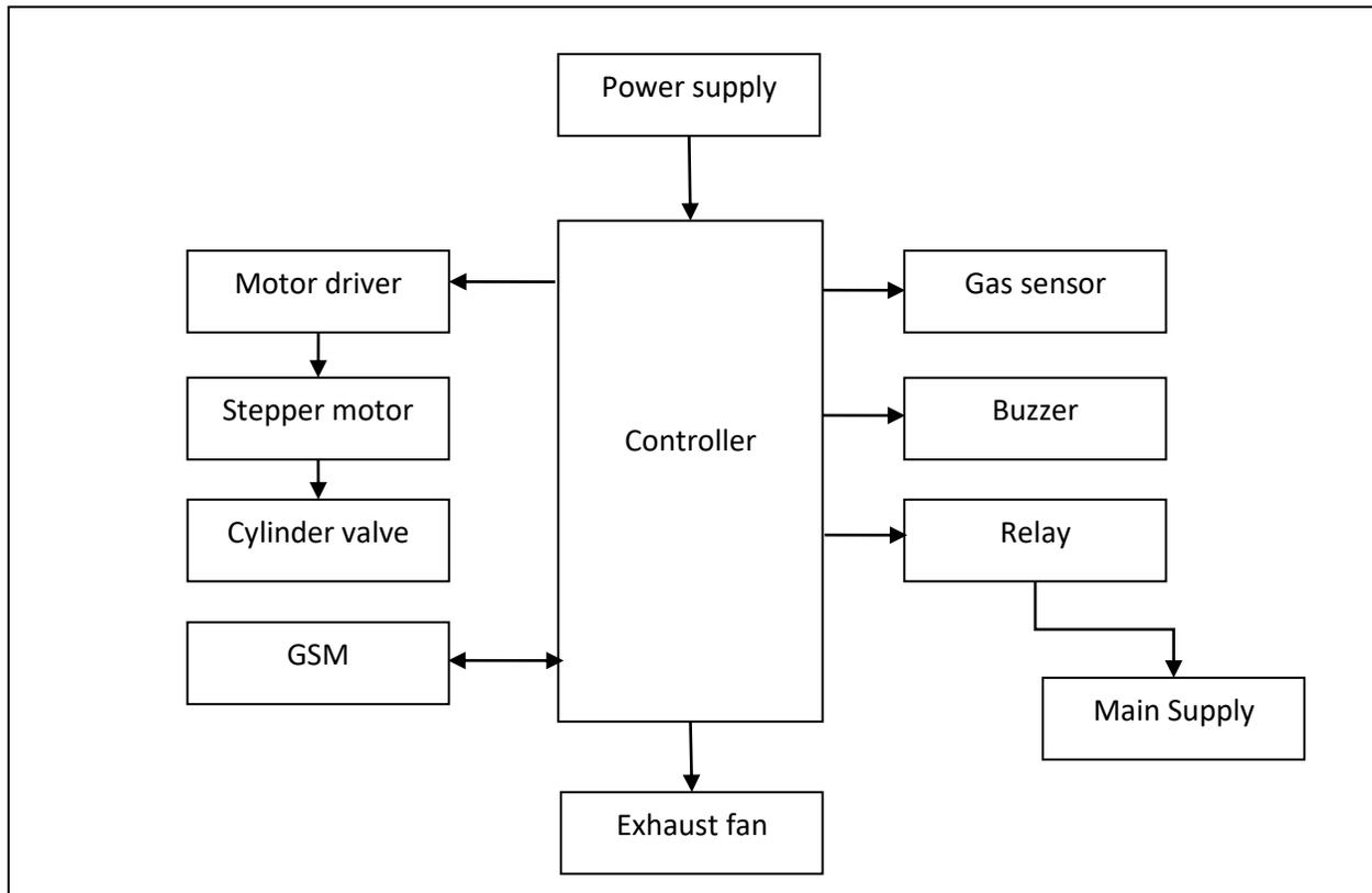
Figure 1: Design of the system
