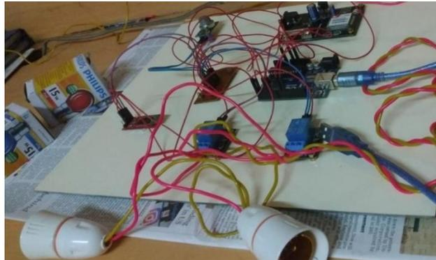
**Figure 2:** Proposed work of smart circuit breaker.
