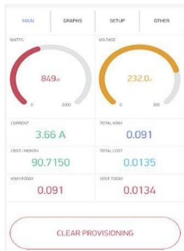
**Figure 3:** Power monitoring using Blynk
