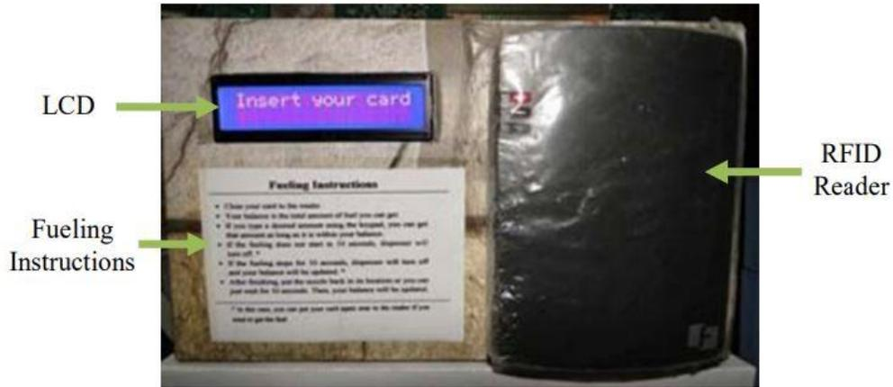
**Figure 3:** RFID reader and hardware module enclosure
