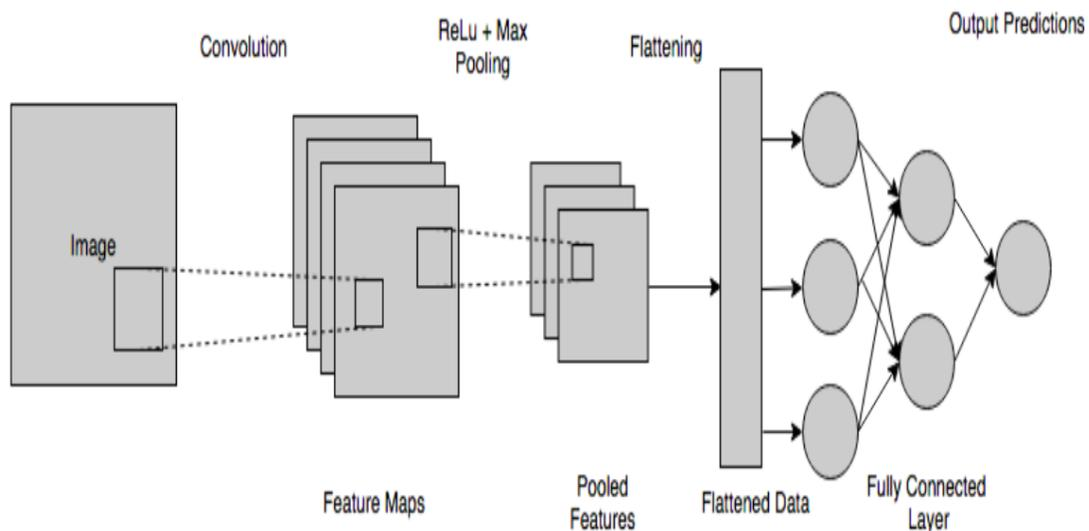
**Figure 2 CNN architecture**
