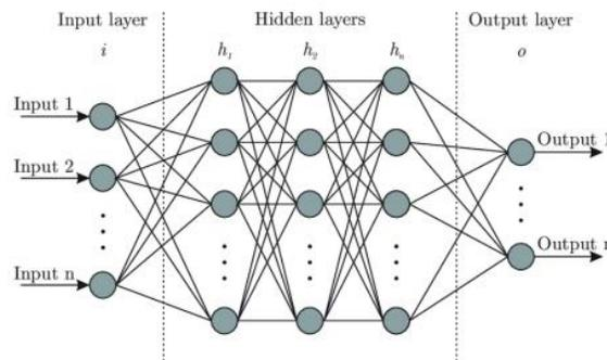
**Figure 4:** ANN architecture (ANN –n level with input, hidden, and output layer).
