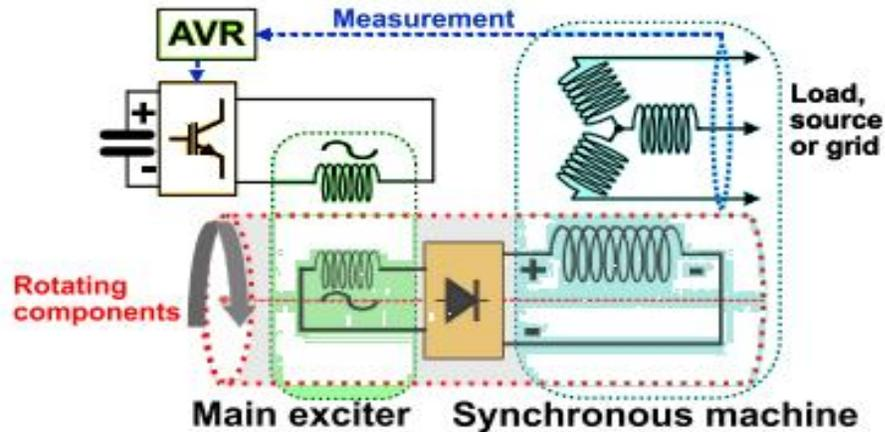
Figure. 4 Rotating transformer
