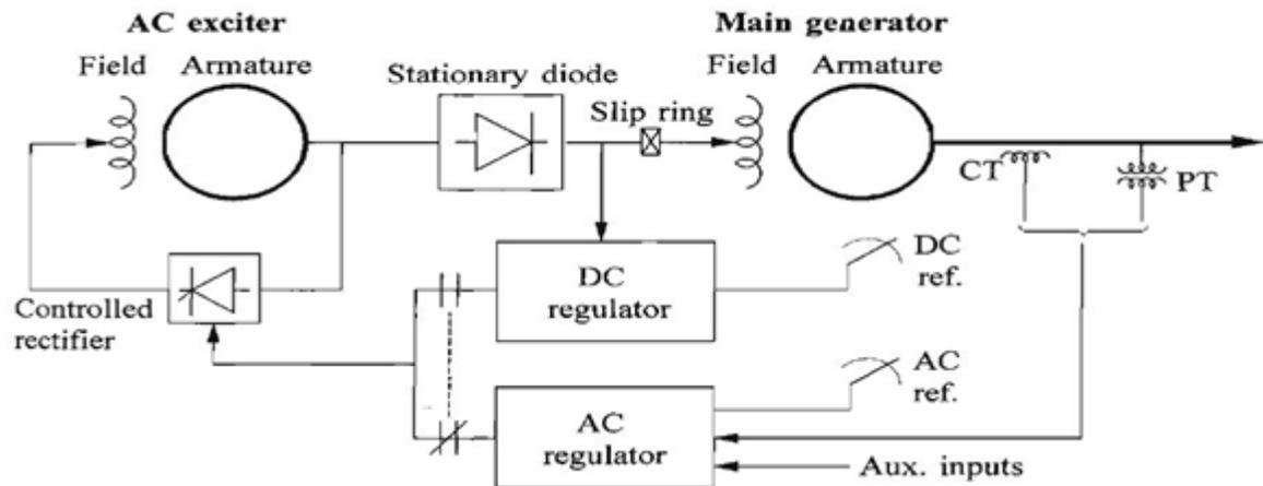
Figure.3 AC excitation systems using DC and AC regulators
