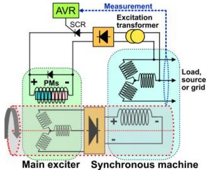
Figure. 5 Shunt hybrid systems
