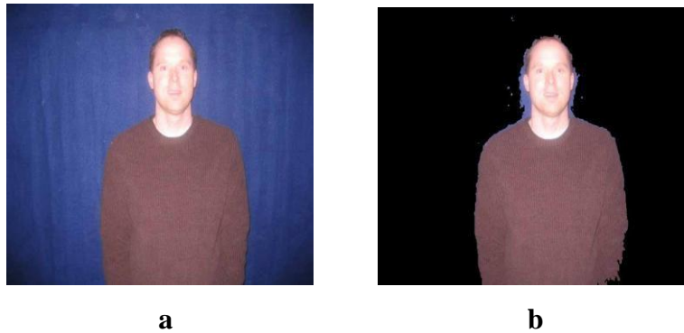
Fig.6 a. Original Image (640 * 480, jpeg, textured) b. Foreground extracted Result
