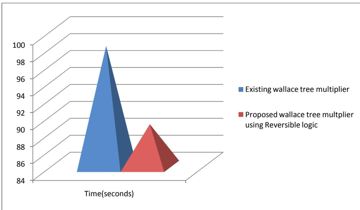
Figure. 6 Delay difference between the multipliers
