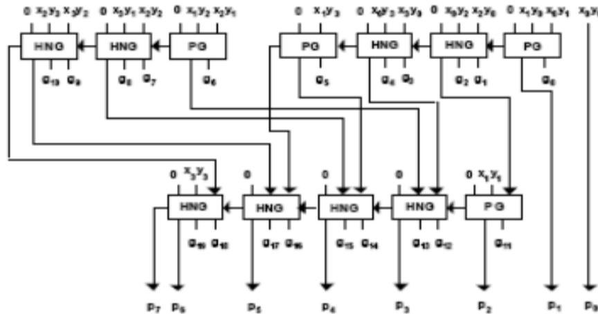
Figure. 2 4-Bit Multiplier using Reversible Logic
