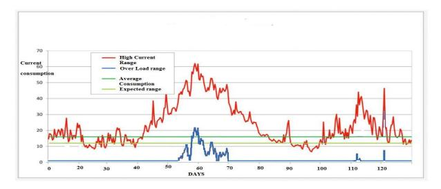
The Graph clearly denotes the current consumption of the motor and also denotes the exact time when the range exceeds (i.e) during the time of overload it has clearly notes. Results:
