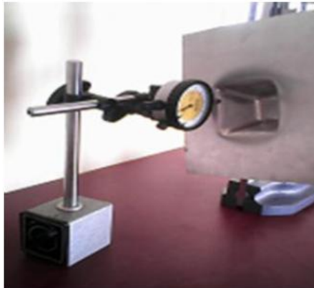
Fig.5 Thinning measurement using Dial
