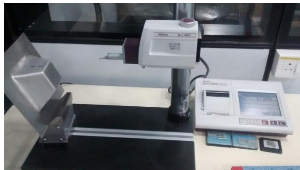
Fig.4 Surface roughness tester taking trace of Ra value
