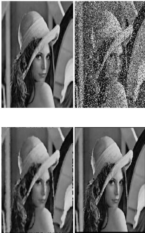
Fig 6. Results of filtering with a 3X3 median and conditional median filter. From left to right, first row: original Image, noisy image; second row: standard median filter, Adaptive median filter.
