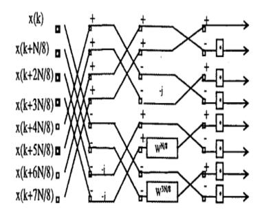
Signal flow graph for Radix-8 butterfly unit. The butterfly unit is designed to perform basically the radix-8 DIF FFT algorithm and also it can compute radix-4 or radix-2 DIF FFT algorithm. It computes the radix-8 FFT in all computational stage.
