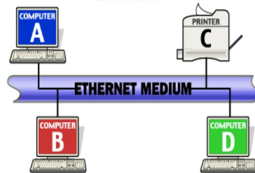
The Ethernet protocol specifies a set of rules for constructing frames. There are explicit minimum and maximum lengths for frames, and a set of required pieces of information that must appear in the frame. Each frame must include, for example, both a destination address and a source address, which identify the recipient and the sender of the message. The address uniquely identifies the node, just as a name identifies a particular person. No two Ethernet devices should ever have the same address.
